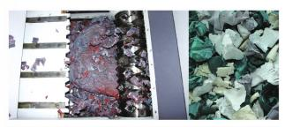
V Series Single Shaft Shredders are small - medium size reduction machines suitable for processing a wide range of materials to a uniform particle size. The output products created can often be sold as is, or be sent for further processing through additional  $equipment \ (granulators \ briquetters \ etc). \ Throughputs \ typically \ range \ between \ 300 kg/hr - 5,000 kg/hr+ \ depending \ on \ the \ machine$ model, material type, screen size and application.
